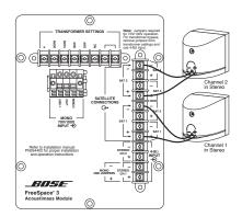
Using 4 satellite speakers with direct connections
