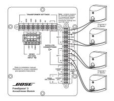
• Using 4 satellite speakers with daisy-chained connections
